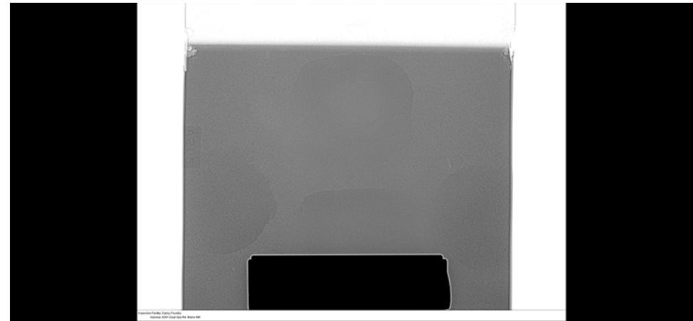
1/2" thick 8"x8" Test Plate X-Ray confirming Grade B
