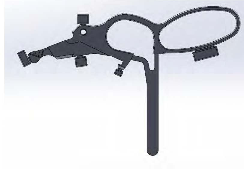
Lever with runner and overflows
