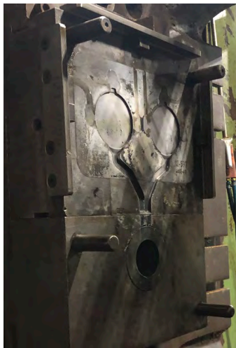
Coaster die on the fixed half of the HPDC machine
