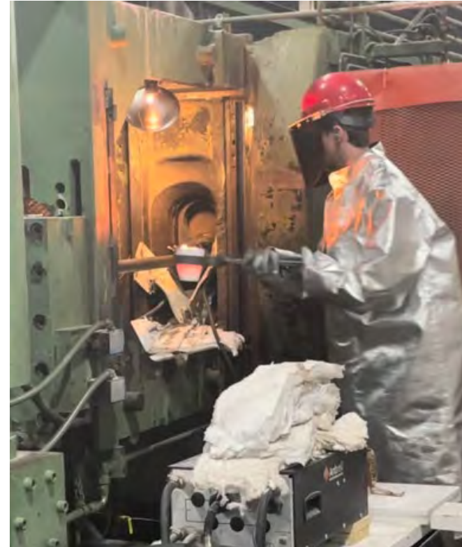
Producing test steel die castings at Mercury's plant in Fond du Lac, WI
