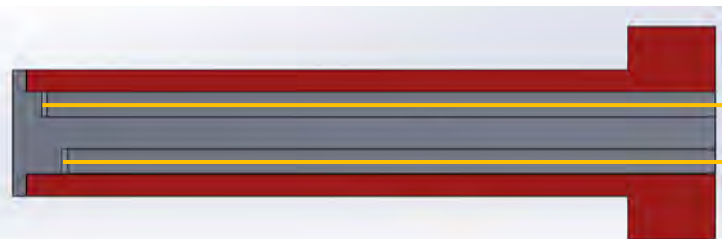
Temperature sensor location in the dies: (a) front view, (b) section view, and (c) runner die front view
