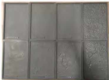
Figure 2-3 Various SCRATA comparators. First row left to right: A1, A2, A3, A4. Second row left to right: B4, C3, D5, E3
