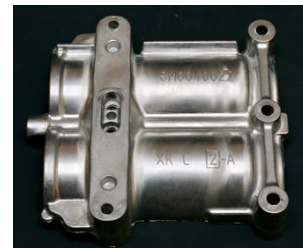
Balance Shaft Housing after more than 70,000 castings have been produced in the die (photograph by Phygen)
