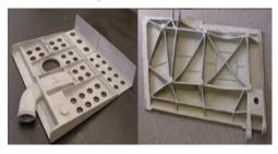
Complex shapes, lofted contours, and ranginess that are common in castings make them more susceptible to distortion during the heat treatment process and therefore require more expertise to correctly heat treat and straighten.
