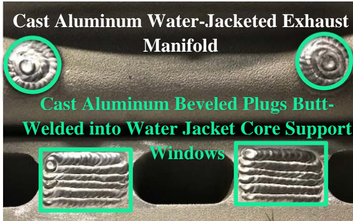
The photo above illustrates the as-welded condition before manual grinding, post-weld heat treatment, and grit blast to smooth the surface per customer requirements.
