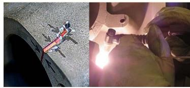
pragmatic approval of in-process weld rework, as one of many normal casting finishing processes, has the potential to drive down the internal scrap rate and the resulting high casting costs and lead times.
