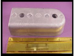
This tank track insert will absorb heat from the rubber, extend track life and prevent strip-off failure.
