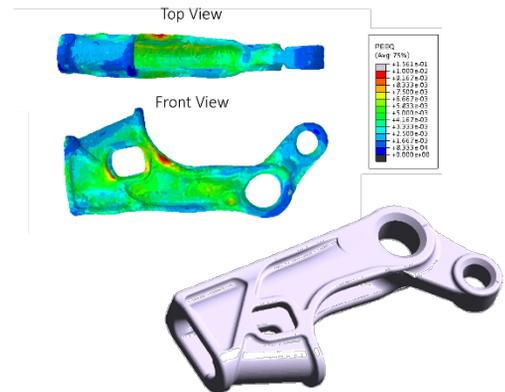
*“The ability to accurately predict as-cast dimensions and distortion through modeling simulation will have a huge positive impact on new product development. Such modeling will help shorten lead times and reduce costs for customers and end users like the DLA by reducing sample iterations, tooling costs and unnecessary machining stock.”*
