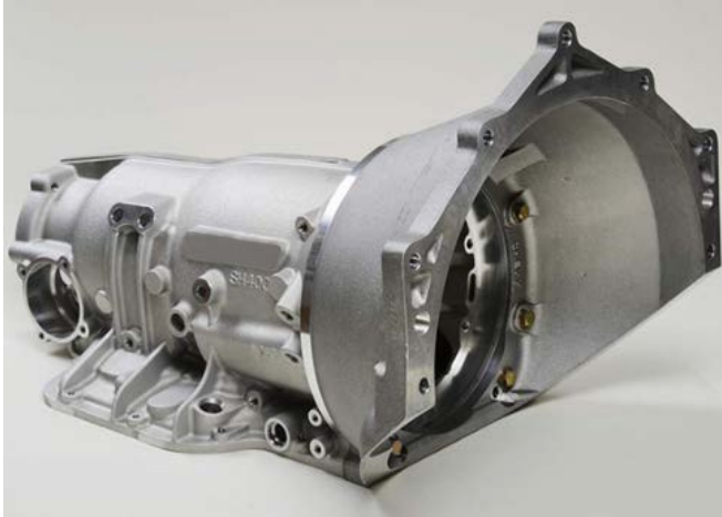
OEM aluminum die cast turbo 400 transmission case. Approximate weight 75 lbs. Courtesy HK AA website. 2
