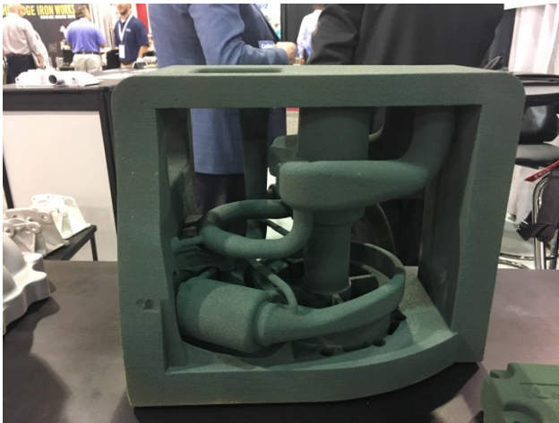
Printed sand one-piece internal passage core assembly for Pump Housing displayed at Cast Expo 2017 1
